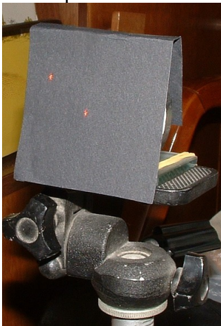
Fig. 18: Angle of the flat is roughly adjusted to put reference beam near the test beam at the mirror under test. The spot on the right is from the test beam.
