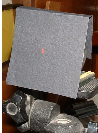
Fig. 20 The flat is rotated about vertical axis for coincidence of two spots.
