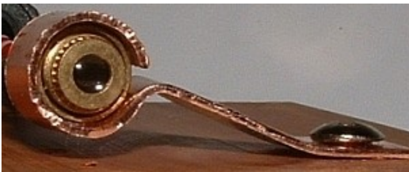
Fig. 10: laser lifted, to have a beam 7 mm above the base
