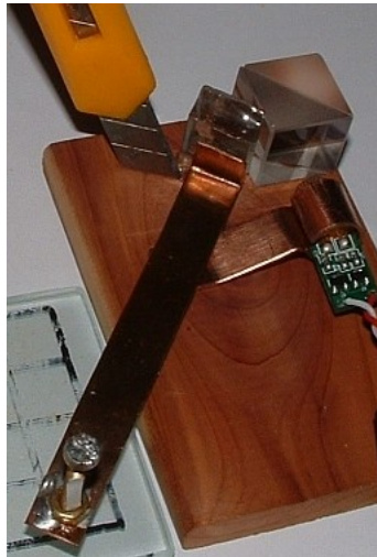
Fig. 21 The adjustment jig is separated from the flat (therefore it was glued to flat lightly),
