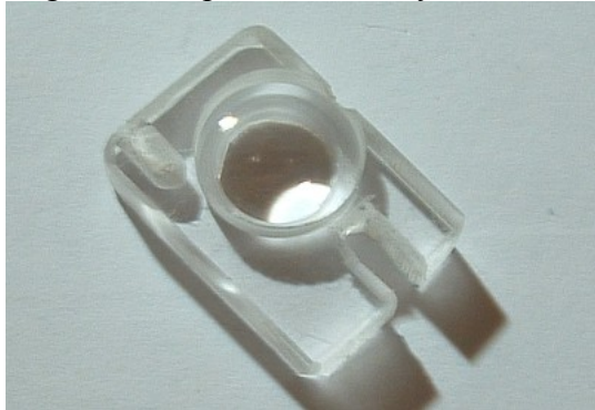
Figs. 23: The lens is inserted in holder, with slot or hole slightly bigger than the screw, to facilitate adjustment in xy plane (up-down, left-right).
