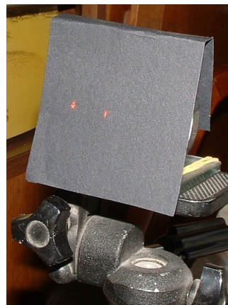
Fig. 19: By adjusting the screw of the jig the flat is tipped about horizontal axis until the reference beam spot is brought to the same elevation
