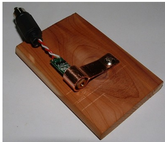
Fig. 9: laser holder screwed to the base. Serves also as a heat sink, if required.
